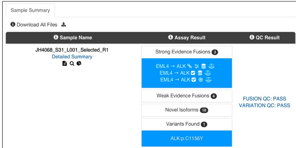
**Figure 25. The result of a targeted mutation shows 1 mutation under the “Variants Found” section for this sample in the ALK gene.**
