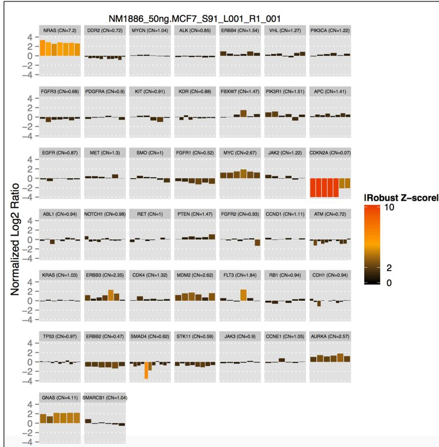
**Figure 37. PDF with the visual representation of the individual target primers for the Copy Number assay. The bar represents the Log<sub>2</sub> value of the normalized copy number ratio (0 = normal for that gene). The color represents the Z-score for the target primer**
